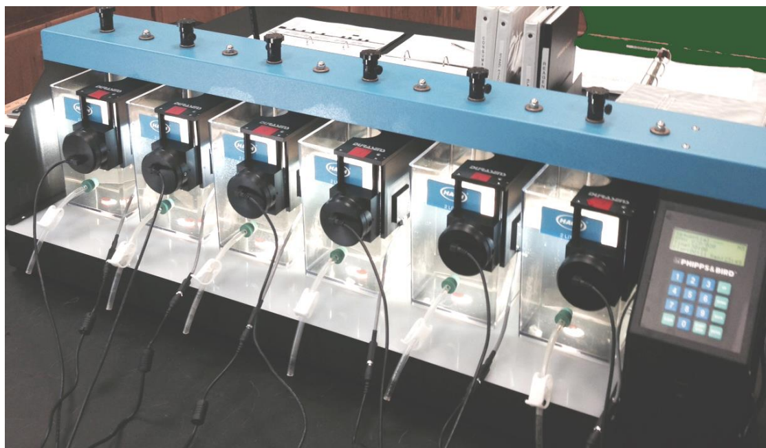
Figure 1: Standard jar test fixture equipped with six Jar FlocCAM®s
